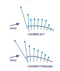
One more factor to consider is that a rounder leading edge or deeper camber, while producing more force, does so at the expense of having a higher entry angle that
