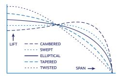
It has been found for an isolated wing in untwisted flow that the spanload with the minimum induced drag is an elliptical distribution of lift. This is achieved on an untwisted, unswept wing with an elliptical distribution of area and the same section along its entire span. A spanload can be altered in several ways.
