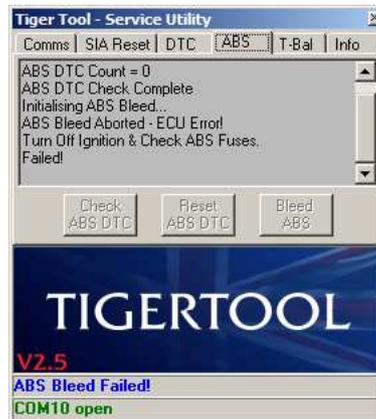
This error can be caused by a faulty supply to the ABS modulator. It usually indicates that the ABS ECU is responding but there's no power to drive the solenoids & pump sections. The ABS fuses and wiring should be checked.
