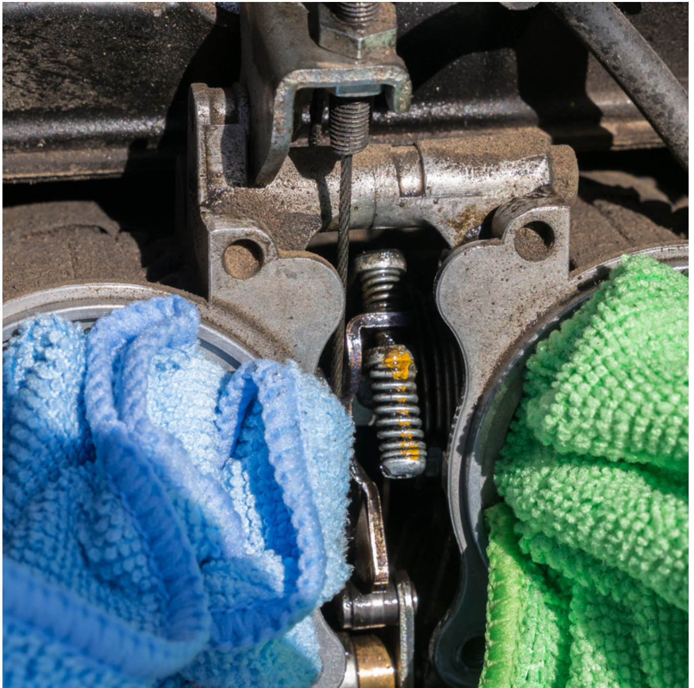
Top of the stepper, throttle linkages and inlets. This whole area gets really dirty, this was a picture from Mexico about 3,000 miles after the last clean. It's the dirt and grime that causes poor idling and stalling.
